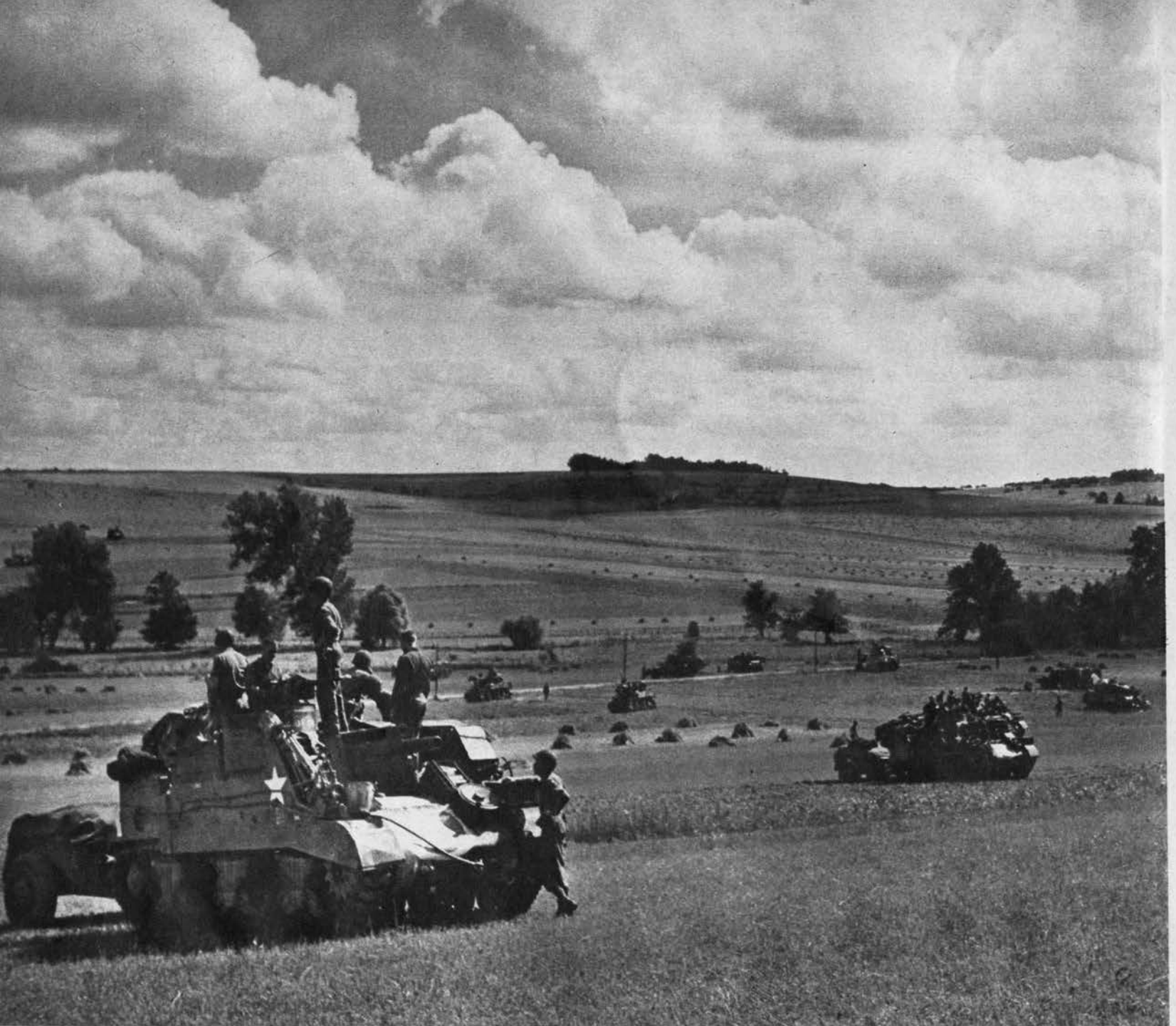
M-7's line up on a French hillside in preparation for an attack on German positions as M-8 SP howitzers and an M-4 maneuver in the background. The M-7 consists of a 105-mm. howitzer mounted on an M-3
